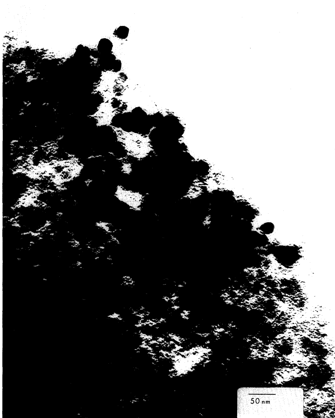
FIG. 9. Transmission electron micrograph of \text{NEt}_4[\text{Fe}_2\text{Mn}(\text{CO})_{12}] catalyst after 16 h reduction at 673 K. Composition, \text{Fe}_2\text{Mn}_{1.26} .
